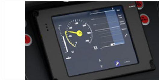
ETCS system GUARDIA (ETCS baseline 3 Release 2) for operation at level 0,1,2 and partially PZB
